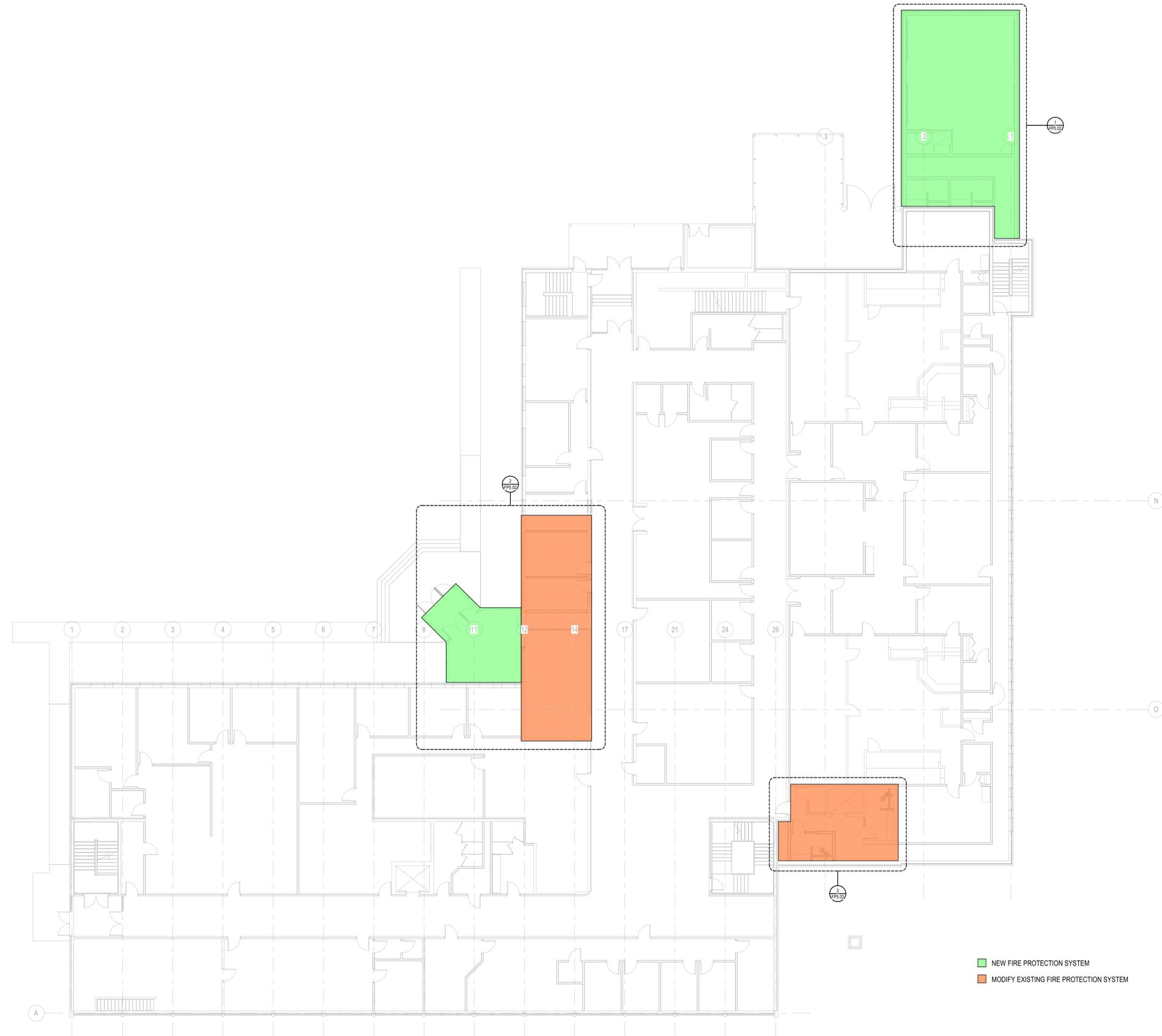
OVERALL FIRST FLOOR FIRE PROTECTION PLAN
