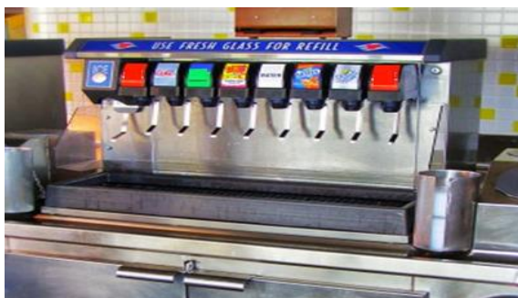
Equipment Sealed to Counter Top
